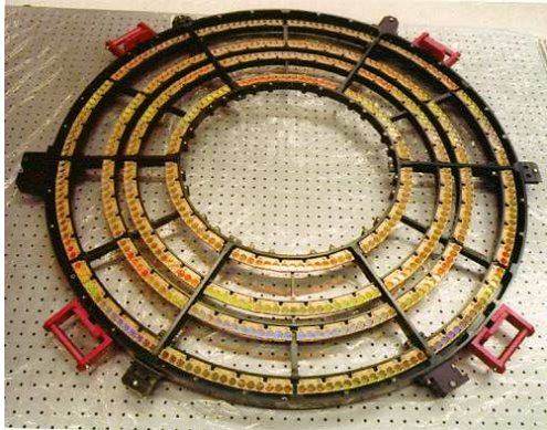
Fig. 8. Chandra LETG grating facets mounted on a toroidal structure upper limit for the He abundance in its photosphere.
